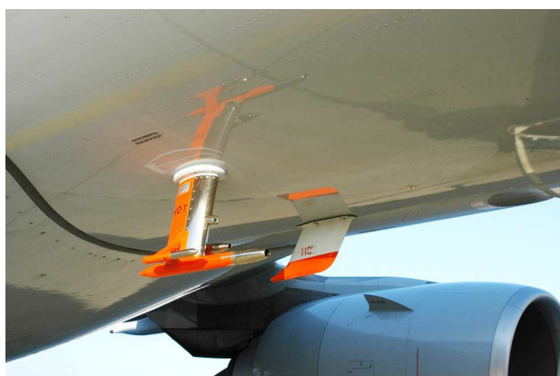
Figure 2. The inlet system as permanently mounted just in front of the belly fairing. The lowermost probe is the aerosol diffuser tube with a leading shroud. Left above it is the trace gas tube. PFA coated tubing is used to transport the air to the container. To the right is the smaller probe for water having a leading orifice (total water) and one at the side (gaseous water). The video camera points slightly downwards. The viewing ports of the DOAS telescopes (one nadir and 2 limb) are just visible on the right side of the main spar close to the skin of the aircraft.
