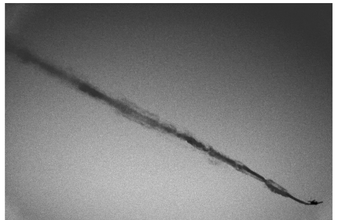
Fig. 2 ATTAS aircraft with smoke-seeded port vortex.
