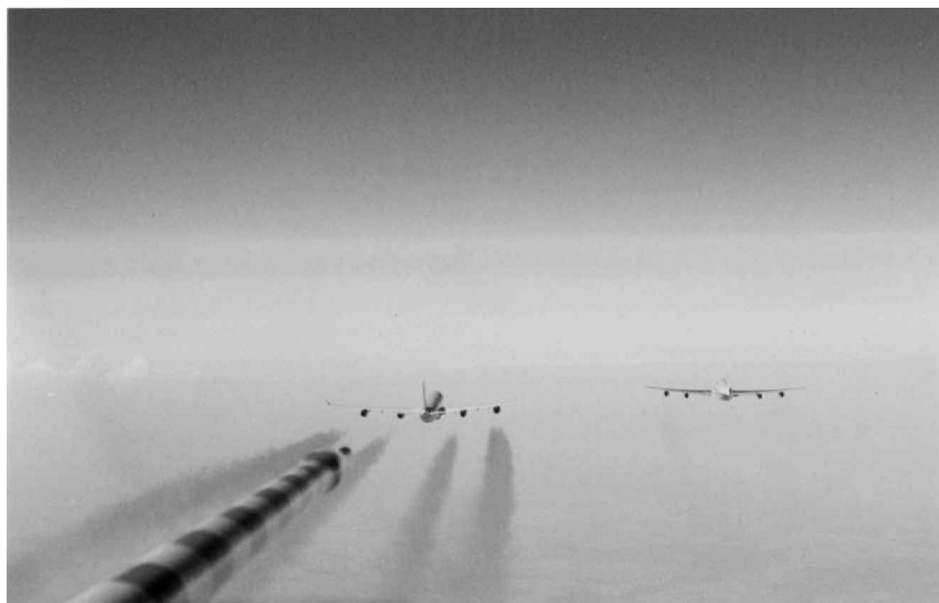
Fig. 3 Airbus A340 with contrails (left) and the Boeing B707 without contrails (right) taken from the Falcon research aircraft at about flight level 344 hft at 7:40 UTC, 15 Sept. 1999.
