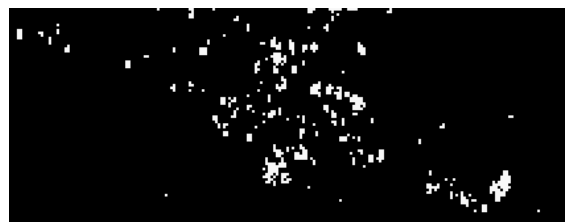
Fig. 5: A map corresponding to the detail image (Fig. 3) indicating where high dynamic data are located (high dynamic =1 (white), low dynamic =0 (black)) in the LH subband.
