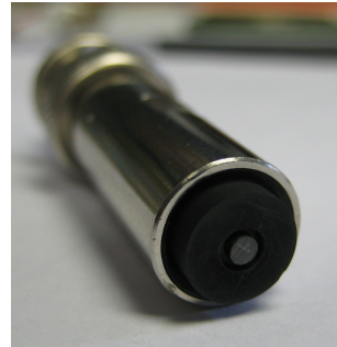
Figure 2.3: The carbon electrodes of the injector head fitted to an SHV clamp connector
