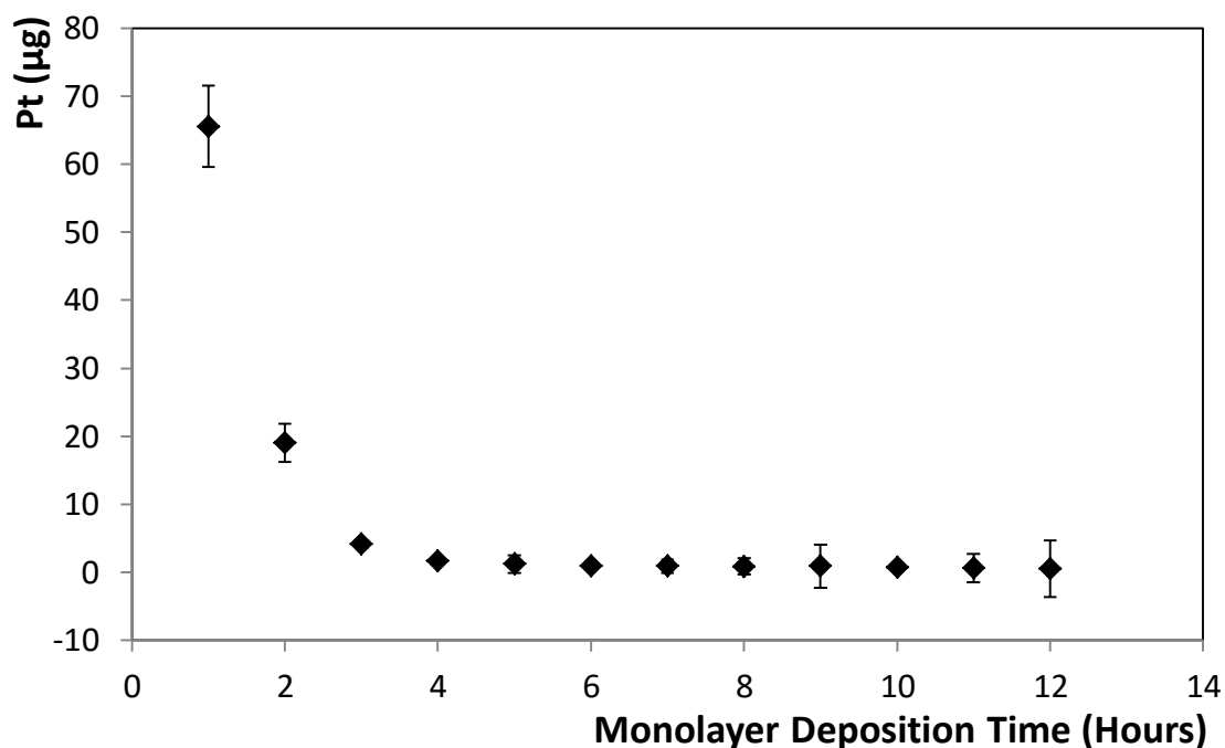
Figure 2.4: Mass of Pt deposited onto 2mm gold electrodes after immersion in a 1 mM solution of dodecanethiol in ethanol between 1 and 12 hours. Applied potential of -0.25V for 180 seconds in 1mM H 2 PtCl 6 in 0.5M H 2 SO 4 .
