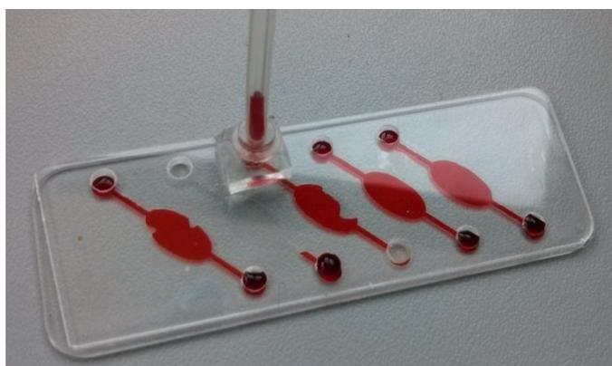
**Figure 6.3: Fluidic device being used in suction mode**
