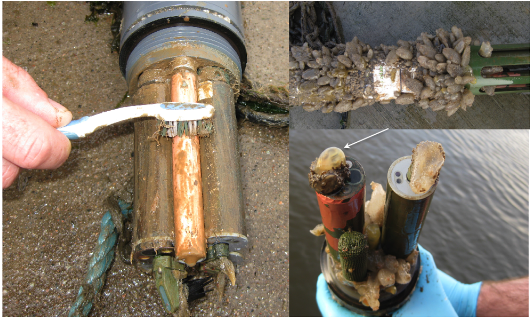
Figure 4.4: An example of biofouling (6 weeks after deployed) on the deployed sensor at Dublin Port during May-June 2013.
