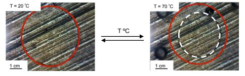
The increase in temperature from 20 °C to 70 °C causes the hydrogels to shrink by  $\sim$ 53% in area.
