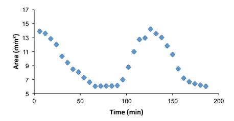
As in the case of salt concentration, the temperature induced shrinking is a reversible, repeatable process.
