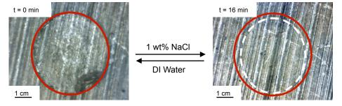
The salt concentration induced shrinking is a reversible process. Changing the hydration medium back to DI water causes the hydrogel to return to its initial size.
