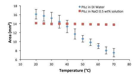
The presence of a chaotropic salt in the hydration solution of the hydrogel inhibits the shrinking caused by the increase in temperature.
