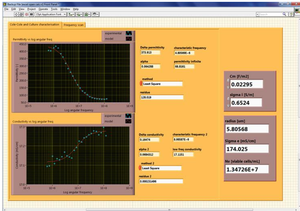
Figure 4.7 Screen shot of a frequency scan undertaken on day 12 of the second perfusion culture, in the RC1. The cell count on that day revealed that the culture had a density of 14.5 \cdot 10^6 cells \cdot mL -1 . The average cell radius measured on that day was 6.2 \mu m
