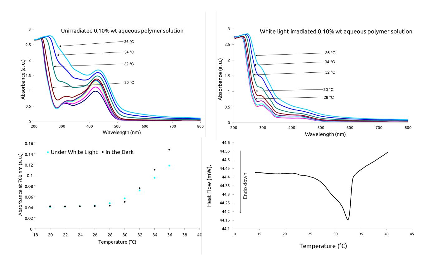
To determine the influence of temperature and white light on the absorbance of the solutions, the temperature was varied between 20 °C and 36 °C, in 2 °C/min steps, either in the dark or under white light irradiation. The endothermic peak which appears at approximatively 32 °C and the increase in absorbance, as seen in the UV-Vis spectra, indicate the presence of the lower critical solution temperature.
