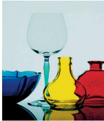
Figure 2-21: Crystal and other types of glassware coated with dye-doped hybrid sol-gel materials[166]
