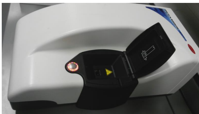
Figure 3-9: Malvern Nano-ZS instrument used for the particle size analysis of the sol-gels.
