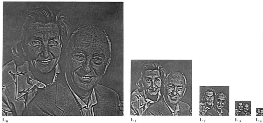
Figure 2.9, A four-level Laplacian Pyramid [21].
