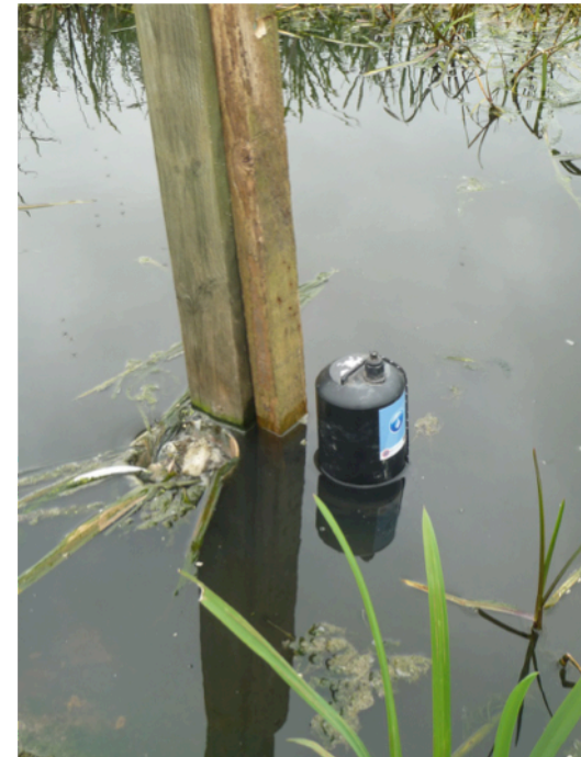
Example of DCU coordinated deployment of autonomous phosphate system in Irish river.
