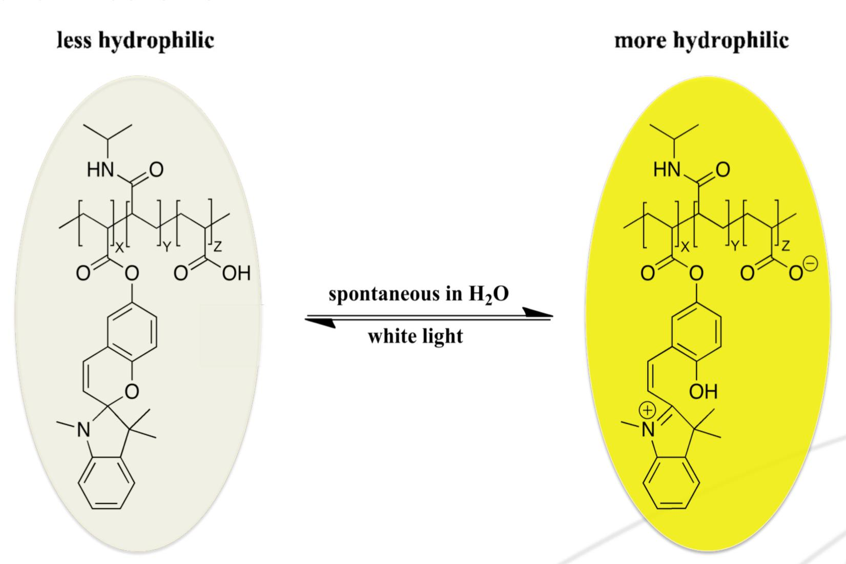
In water, the acrylic acid comonomer dissociates, resulting in the protonation of the photochromic spiropyran (SP) to protonated merocyanine (MC-H<sup>+</sup>). This form is hydrophilic allowing the hydrogel to swell. Exposure to the white light promotes isomerisation of MC-H<sup>+</sup> form to the less hydrophilic SP form, triggering the hydrogel to contract.
