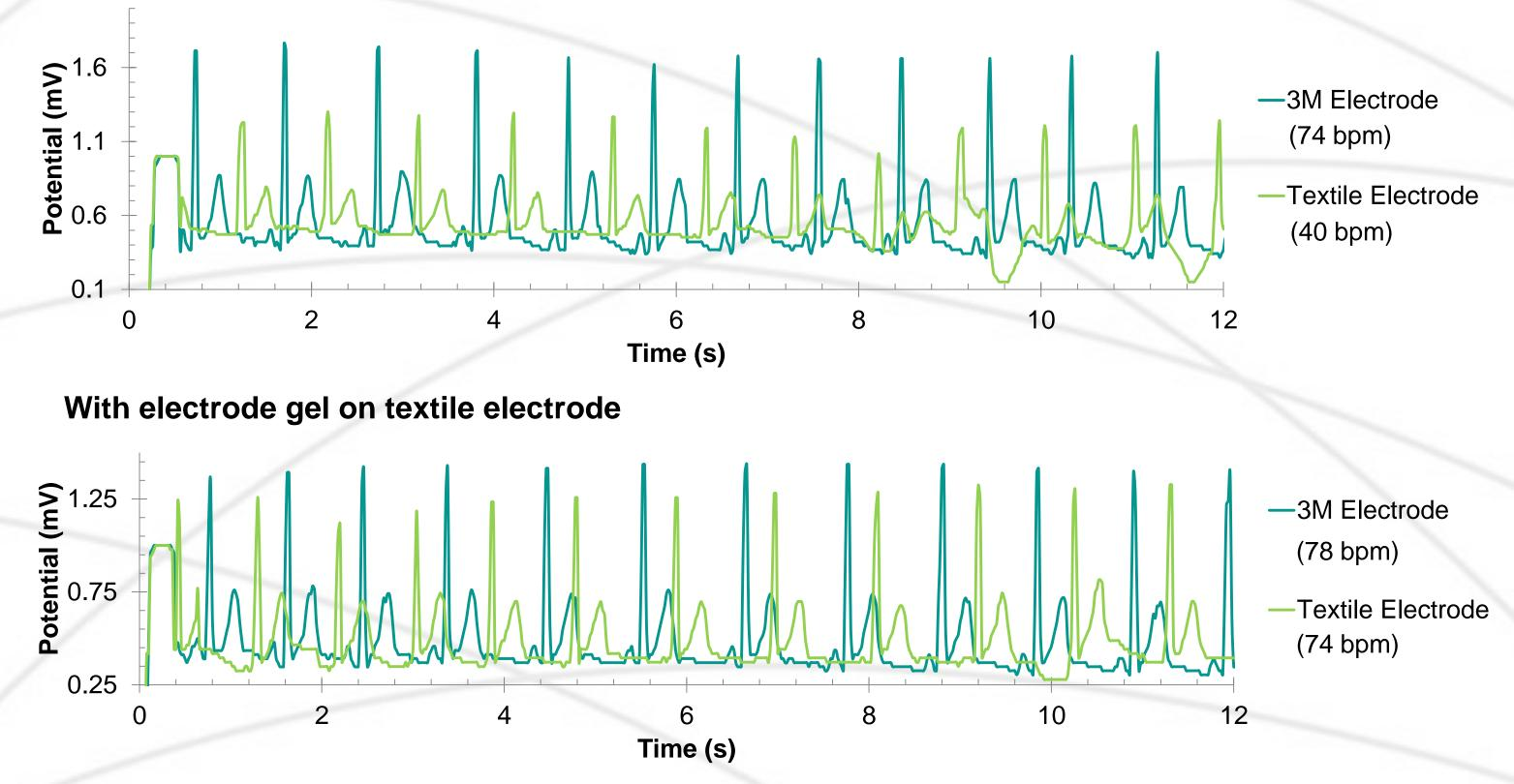
Resting ECG measurements were taken on a healthy adult male with both electrodes simultaneously. Without electrode gel, the textile electrodes showed erratic behavior, with sudden increases and decreases in heart rate that were not present with the 3M electrodes.
