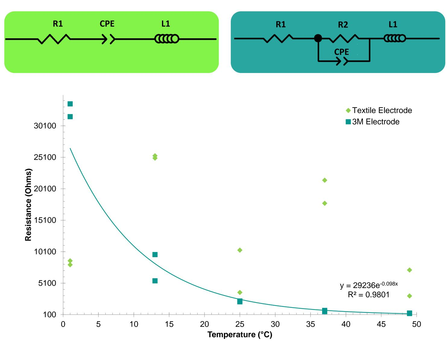
Standard Ag/AgCl disposable monitoring electrodes rely on the well known AgCl +  $e^- \leftrightarrow$ Ag + Cl<sup>-</sup> reduction-oxidation reaction to produce clear, reliable
