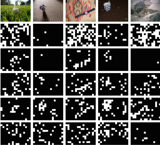
Figure 7: Binary masks after thresholding the EEG maps. The top row is the original images and the remaining rows are the binary masks for five different participants.
