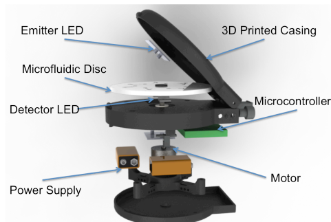
Fig. 3: Computer generated exploded view of the CMAS components
