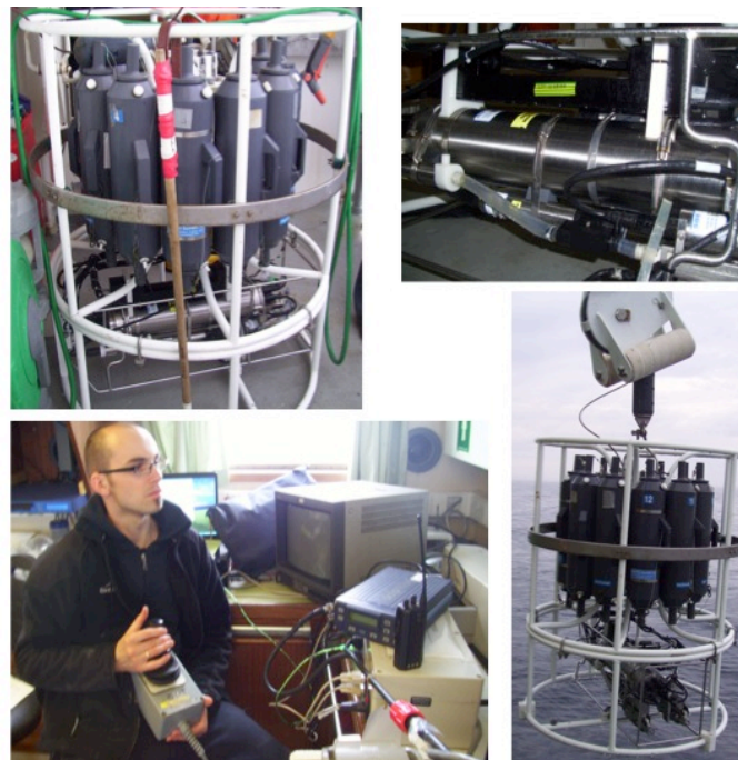
Figure 6: Sea-Bird 9plus CTD profiler (Clockwise from top-left) 1) Rosette sampler close-up 2) Sensor system close-up 3) Deployment 4) Remote operation
