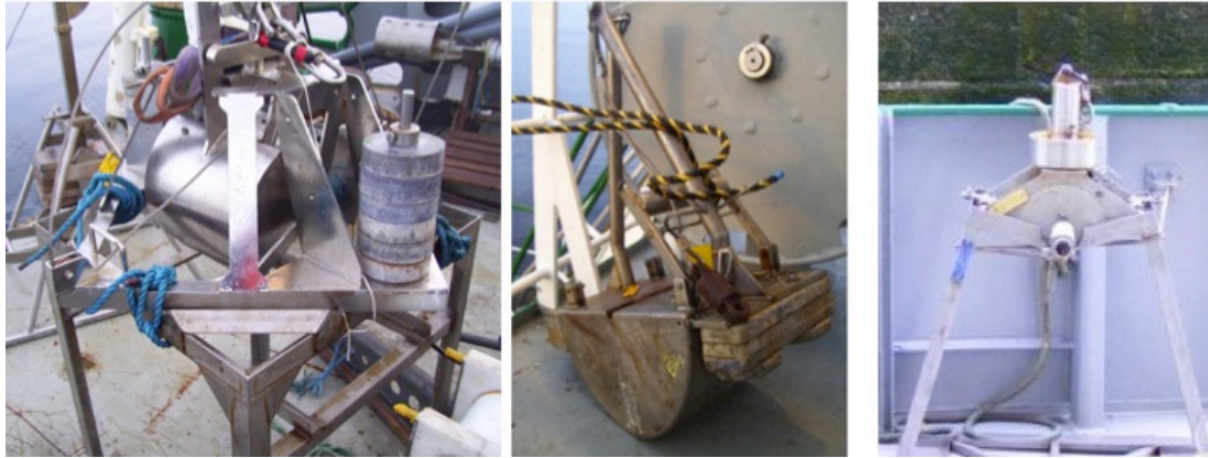
Figure 1: Grabs used on cruise (From left) 1) Day grab 2) Van Veen grab 3) Shipek grab
