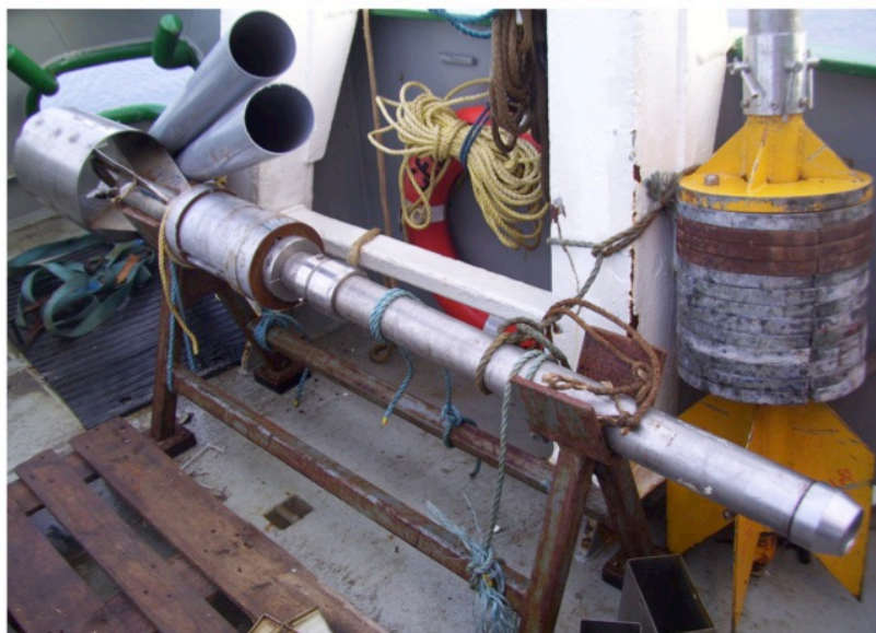
Figure 3: 1m gravity corer (with 2m gravity corer on right)
