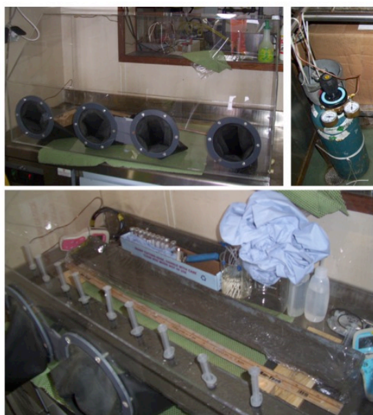
Figure 8 : Custom-built glove box (Clockwise from top-left) 1) Glovebox 2) Argon supply positioning 3) Measuring volatile and redox sensitive parameters
