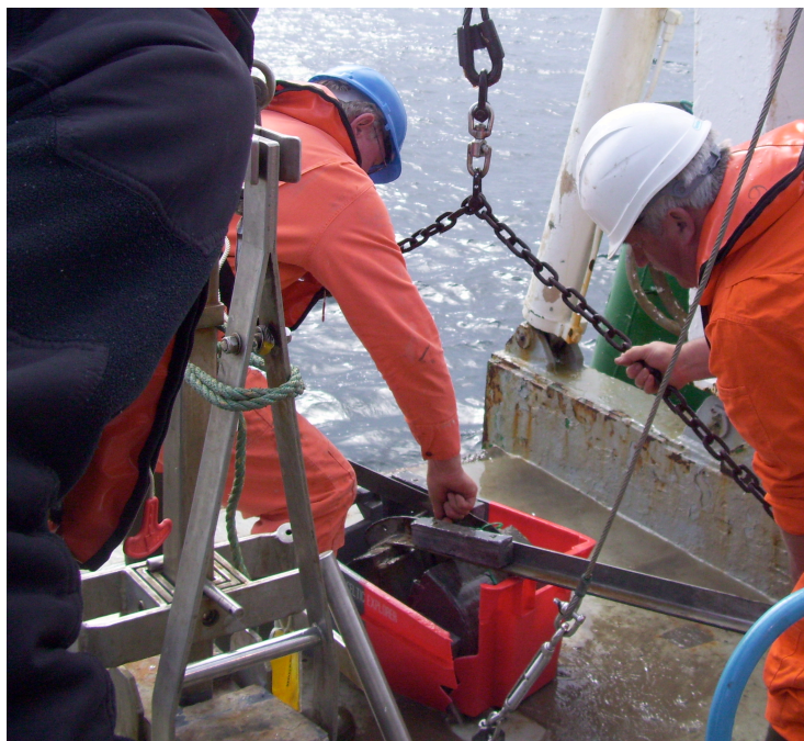
Figure 17: Sampling of MDAC at the Codling Fault Zone, here using the Van Veen grab
