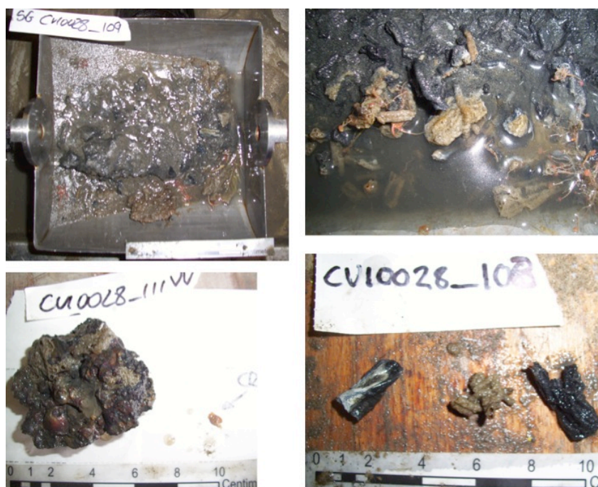
Figure 18: MDAC ground-truthing. (Clockwise from top right) 1) Successful recovery of MDAC using Shipek grab 2) Close-up of highly anoxic sediment, cemented shells and plant-like organism 3) Close-up of large 7cm MDAC nodule 4) Close- still if numerous varying types of hard MDAC fragments and cemented shell tubes.
