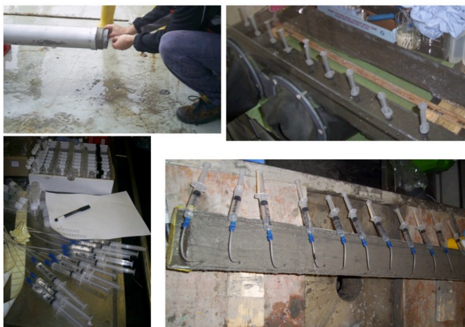
Figure 9: Vibrocore and gravity core processing (Clockwise from top left) 1) Gas sub-sampling of core catcher 2) Gas sub-sampling and redox measurements 3) Porewater sampling 4) Porewater sub-sampling and preservation
