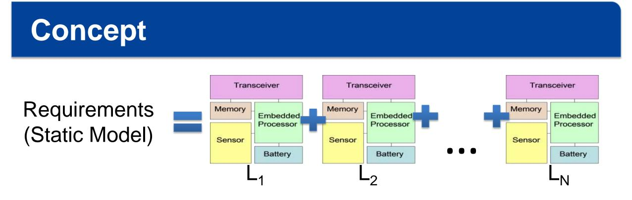
The *static* distributed sensing model requires a number of individual components per location/device (above). By encapsulating most components within a single device and placing the chemo-responsive sensor at designated locations (below), a more cost effective model is achievable. The common components are embedded within a moveable platform giving rise to a *dynamic sensing* model.
