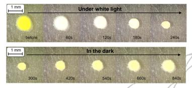
The hydrogels can reach ~49% of the fully hydrated size after 4 min of white light irradiation. After the removal of the white light the hydrogel reswelled up to ~91% of the fully hydrated size after 11 min in the dark. This shrinking and re-swelling cycle can be repeated with great reproducibility.
