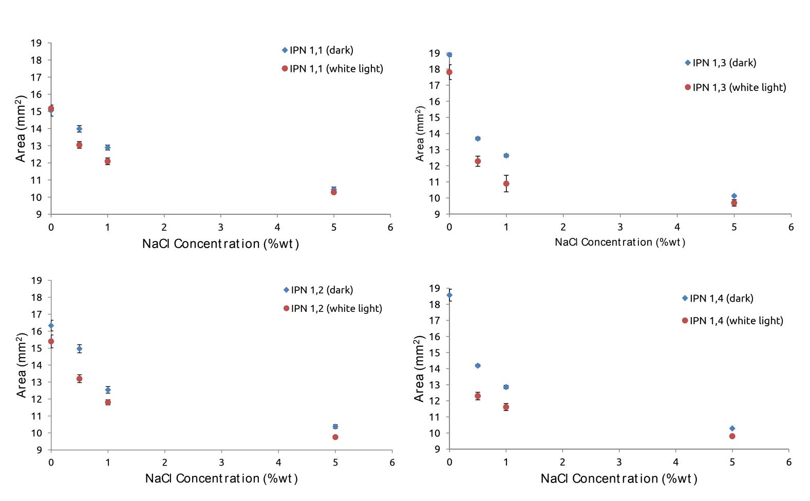
The size of each hydrogel was studied before and after white light irradiation (30 minutes) in the presence of deionized water and NaCl solutions (0.5 wt%, 1 wt% and 5 wt%). For each gel a series of three pictures were taken with a digital microscope, followed by measuring the area five times for each picture.
