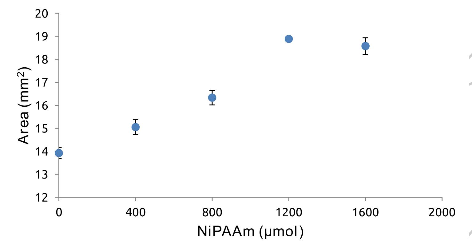
The area of each sIPN was measured after hydration in deionized water for 18 hours.
