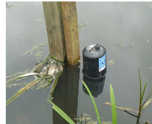
Example of DCU coordinated deployment of autonomous phosphate system
