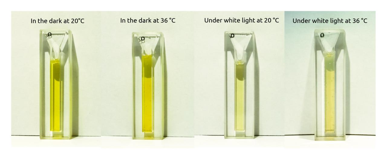
These photos show a 0.10% aqueous solution of the polymer under different temperature and lighting conditions.
