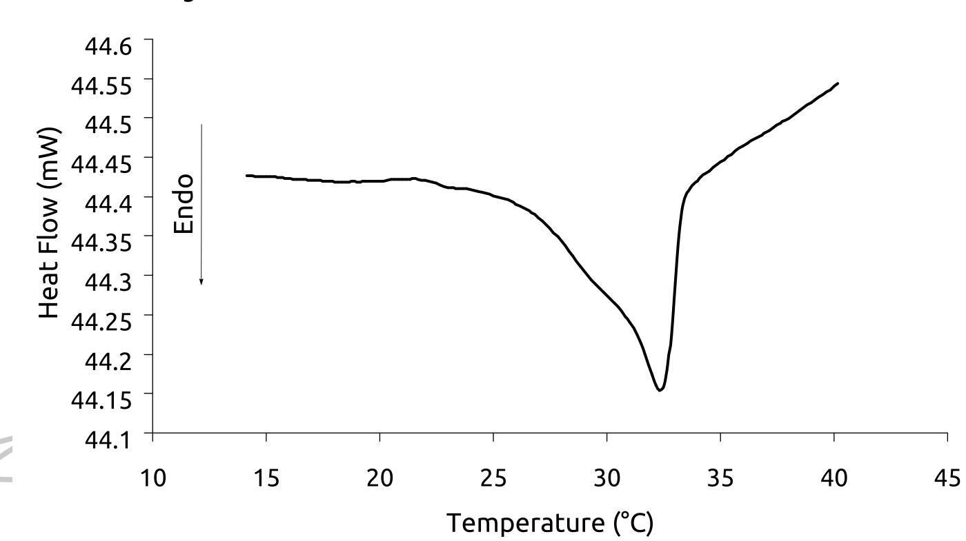
The endothermic peak which appears at 32 °C confirms the existence of a LCST temperature. The scanning interval was from 14 °C to 70 °C at a scan rate of 10 °C/minute.
