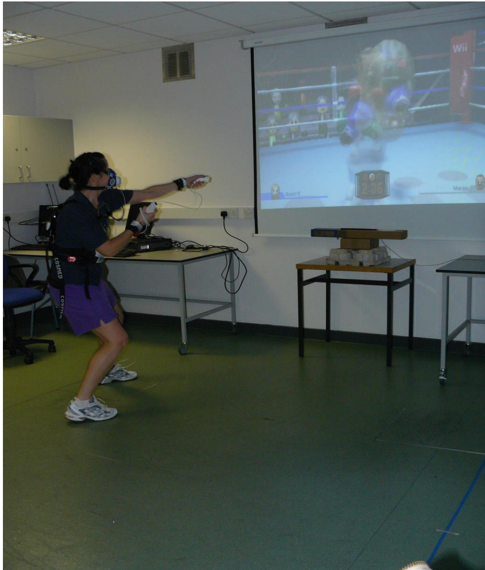
Figure 3.2. Research participant wearing the Cosmed K4B2 and playing one of the AVGs.
