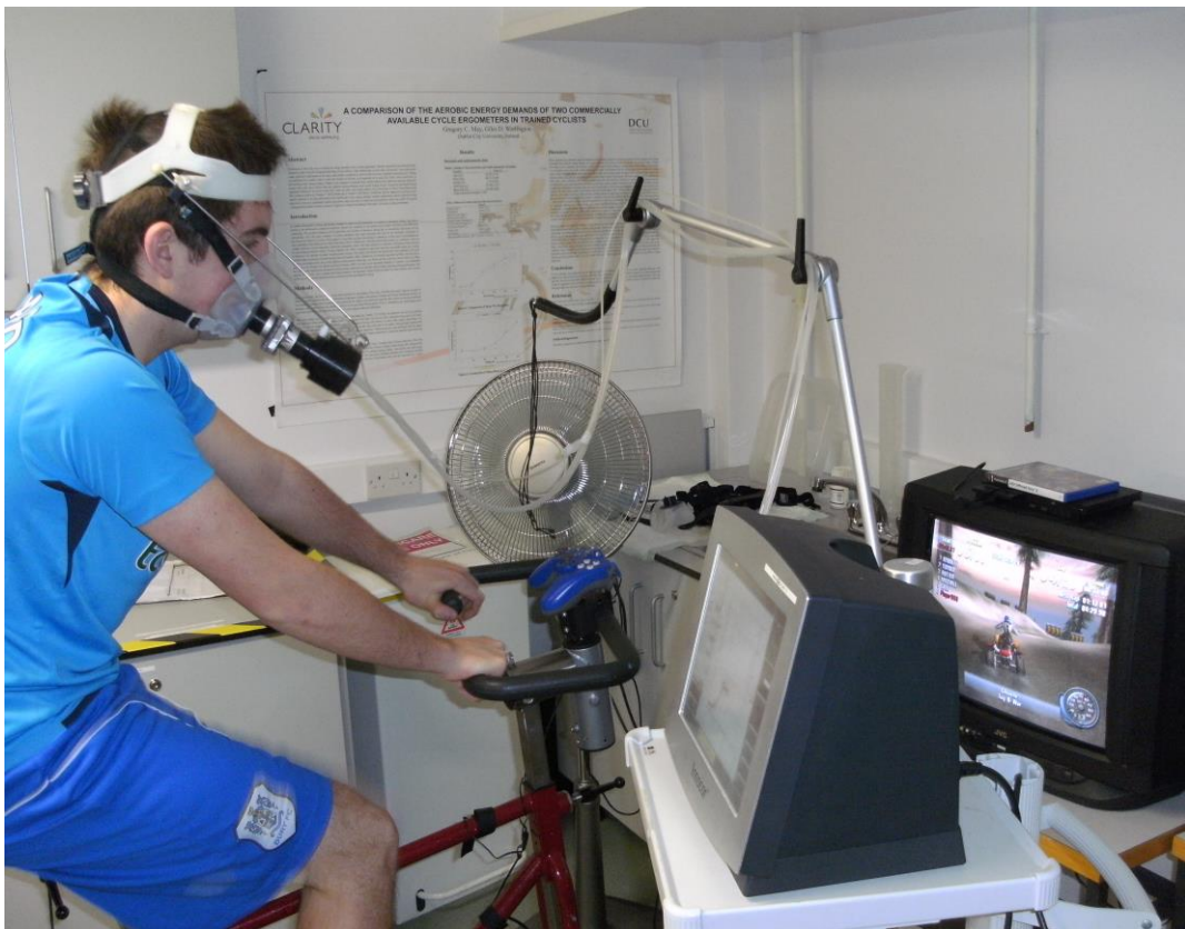
Figure 4.2. Research participant playing GameBike in the adapted Velotron ergometer and wearing face mask for open-circuit spirometry analysis.
