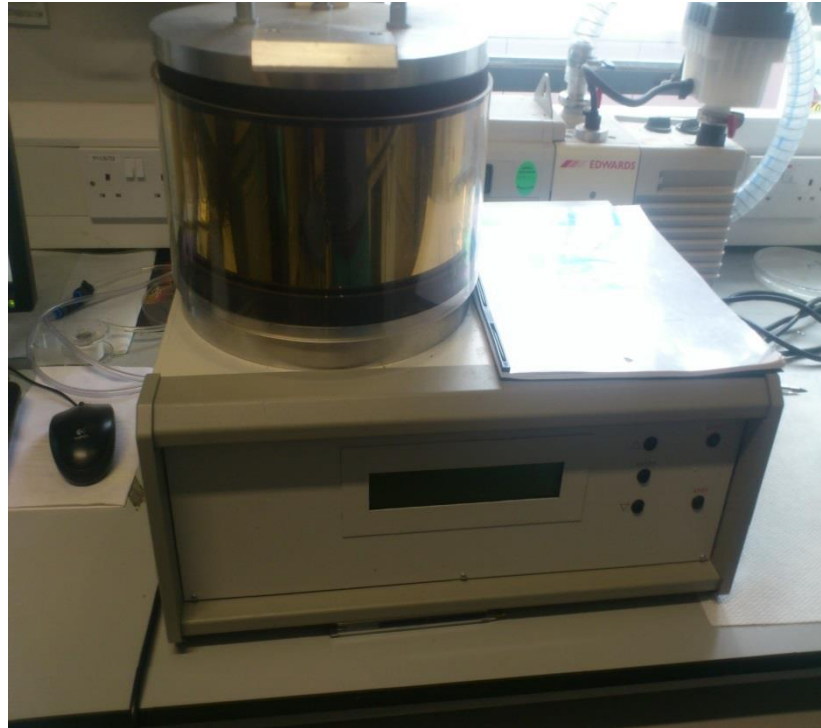
Figure 2.5: Photograph of gold sputter-coater apparatus.
