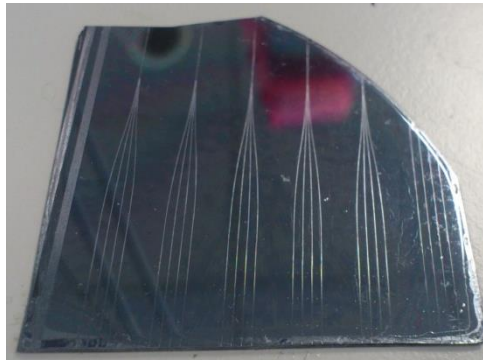
Figure 3.49: Series of diverging 10:2.5:0.25 hybrid sol-gel waveguides on a buffer layer of 10:2.1:0.25 sol-gel materials.
