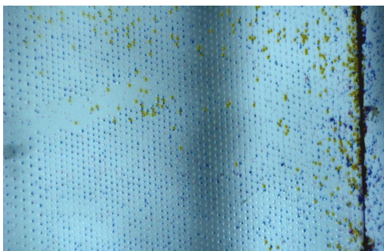
Figure 3.13: Image of 6\mu\text{m} , 10\mu\text{m} and 15\mu\text{m} cups (right to left) and occupancy of 5\mu\text{m} (red), 10\mu\text{m} (blue) and 20\mu\text{m} (yellow) beads. 20\mu\text{m} beads get trapped at various points on the assay but only a very limited number reach the 20\mu\text{m} cups. The 20\mu\text{m} , 10\mu\text{m} and 5\mu\text{m} cups are occupied with a mixture of 10\mu\text{m} and 5\mu\text{m} beads, with most cups filled with a number of beads.
