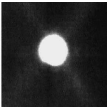
Figure 3.50: Near field image of 1.55\mu\text{m} light output from a 7\mu\text{m} \times 7\mu\text{m} rectangular zirconium sol-gel waveguide [197]. This image is similar to that obtained in this work using a coupling wavelength of 625nm light into 6\mu\text{m} \times 6\mu\text{m} waveguides.
