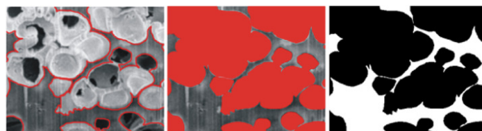
Fig. 4 From L to R: Outline of the pores, filling of pores and binarisation applied to the image stack obtained for the carbon monolith.
