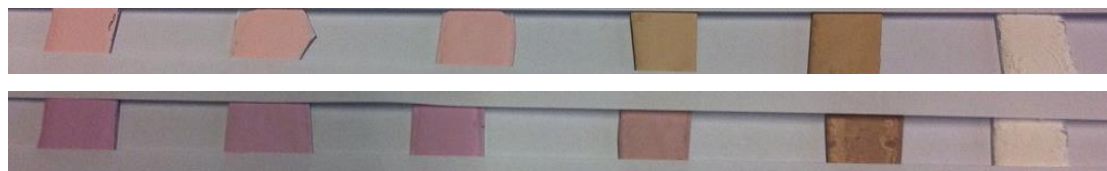
Figure 4.12: Photo showing samples of zeolite-complex materials drop coated onto glass slides. The top shows Z-[Ir(bpy) 3 ] 3+ samples with increasing complex concentration. The bottom photo shows Z-[Ir(bpy) 3 ] 3+ with increasing concentration. In each case the slide at the far right is zeolite-Y with no entrapped species.
