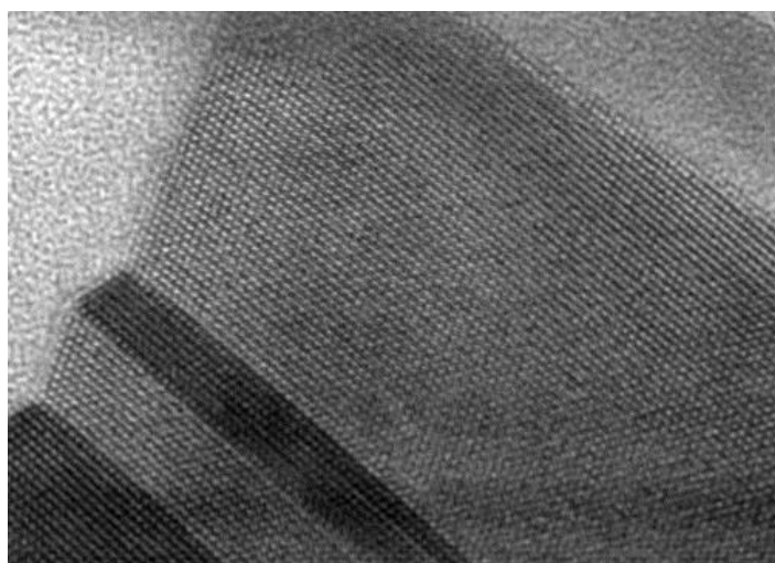
Figure 1.7: Zeolite-Y looking down [011] direction as observed by Wang et al. ( J. Nucl. Mater. 2000, 278, 233). 37
