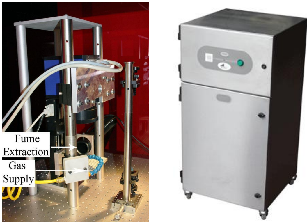
Figure G-9 Gas supply and fume extraction assembly.
