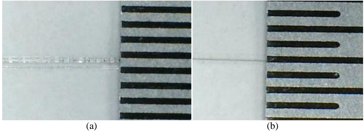
Figure 6-16 Microscopic images of microchannels cut with (a) laser ablation (b) xurography
