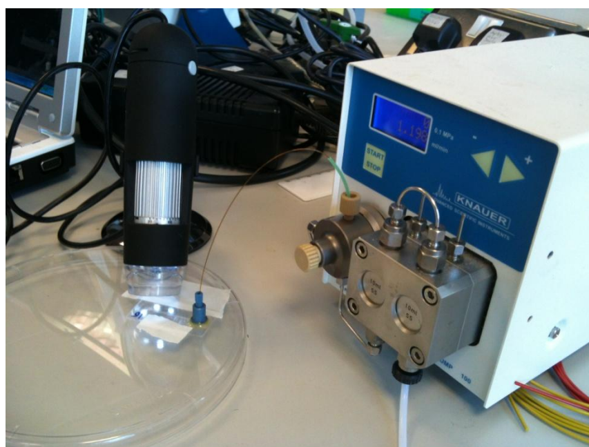
Figure 6-12 Photo of the back-pressure measurement set up
