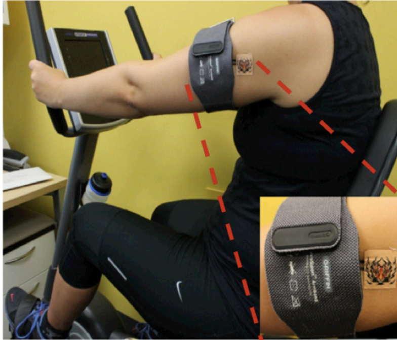
Figure 2. 5: Example of a wearable sensor for sweat monitoring: skin tattoo connected to a bluetooth electronic platform for sodium monitoring (adapted from reference [76]).
