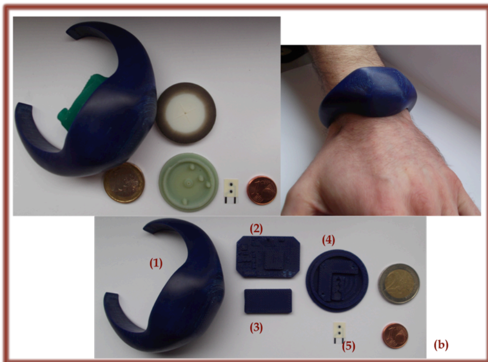
Figure 8. 3: (a) First generation design of the wearable system used to monitor \text{Na}^+ variations, with all the components constituting the device. (b) Second generation miniaturised design with a watch-like configuration where all the different components are disclosed, characterised by new shapes and sizes: (1) 3D-printed encasing with a watch-like design; (2) 3D-printed electronic circuit board; (3) battery sizes; (4) sweat collector and microfluidic design integrated on top of the (5) screen-printed electrodes.
