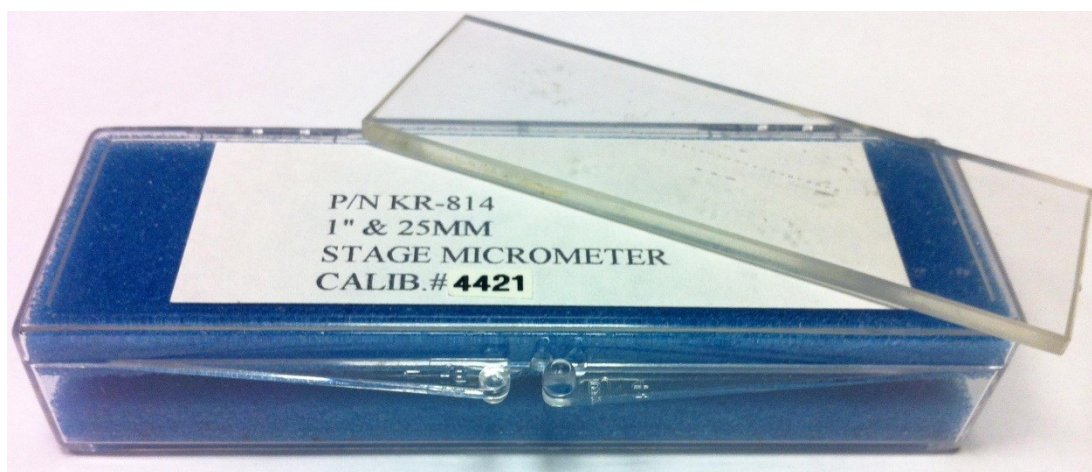
Figure 6-12: The utilised stage micrometre.
