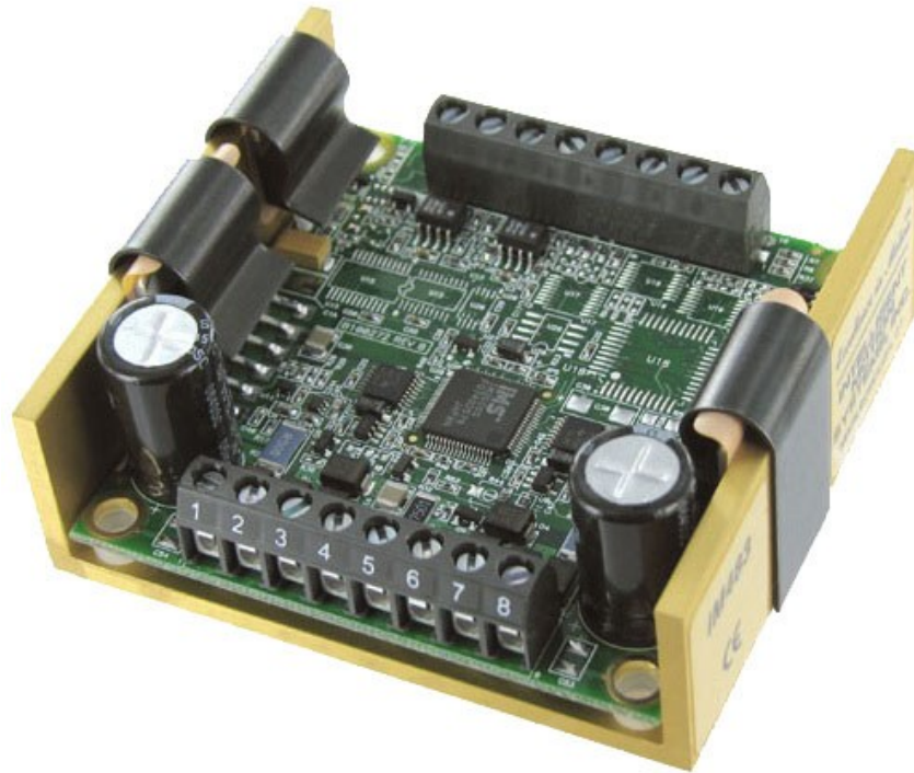
Figure 6-5: The IM483 Micro-stepping Stepper Motor Driver.
