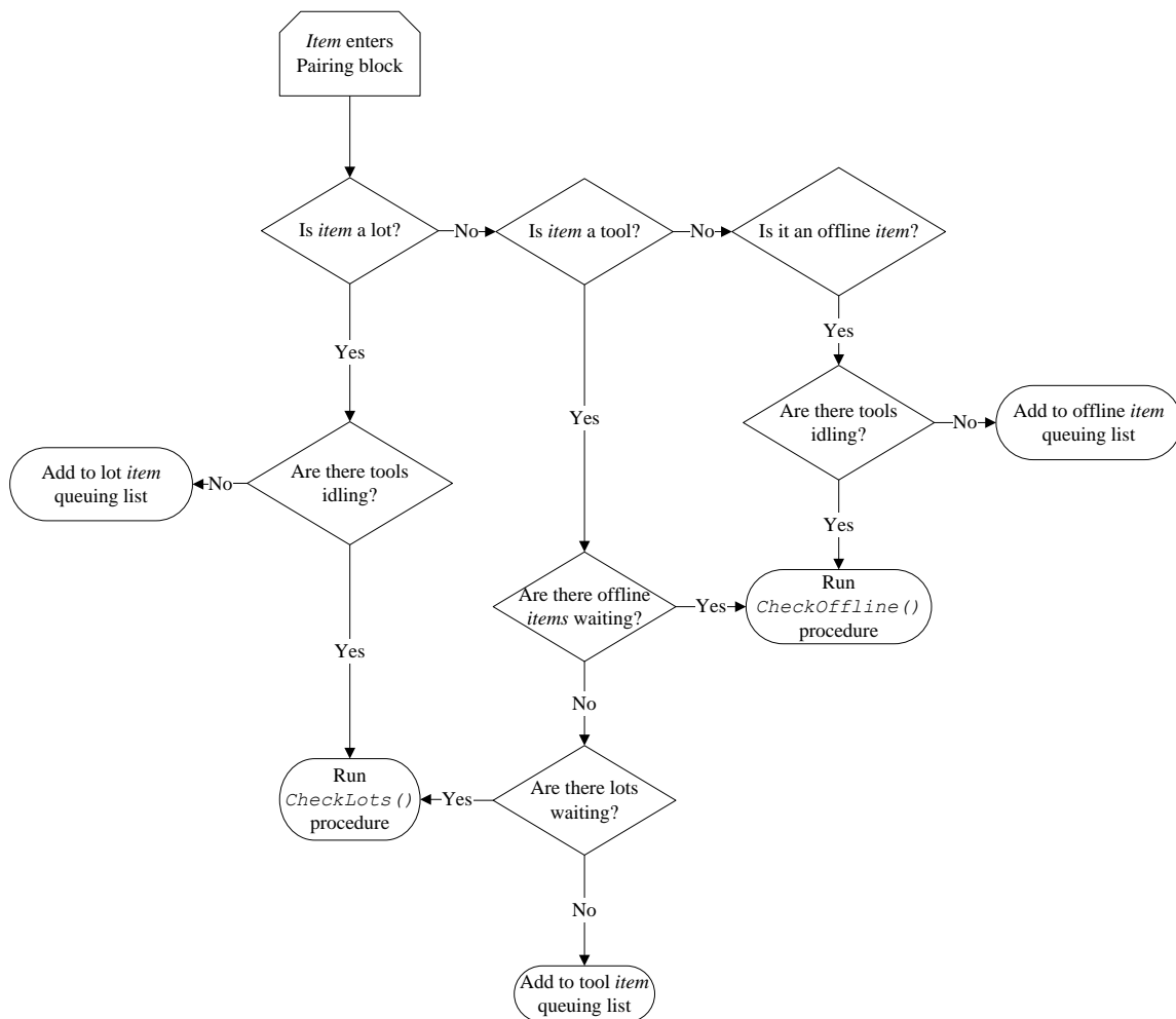
Figure 4.18: Logic code execution for Pairing block used in the FTM application.
