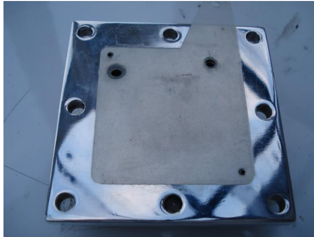
Figure 302 Gasket placed on backing plate.
