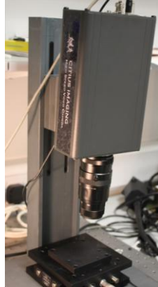
Figure 73 High speed camera set up.
