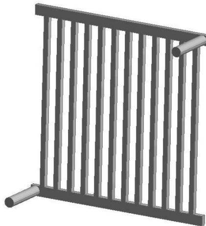
Figure 84 Modified parallel flow plate design with 2mm ribs.
