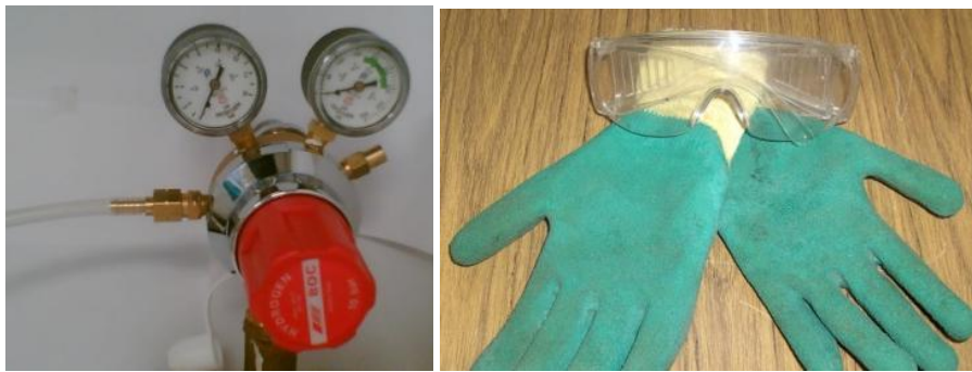
Figure 69 Hydrogen rated fittings and safety equipment.
