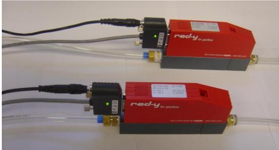
Figure 59 Hydrogen & Oxygen/Air flow meters/controllers.
