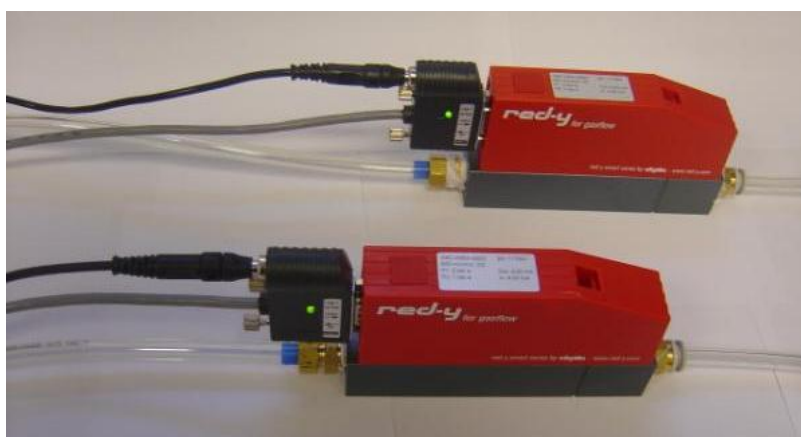
Figure 323 Hydrogen & Oxygen/Air flow meters/controllers.
