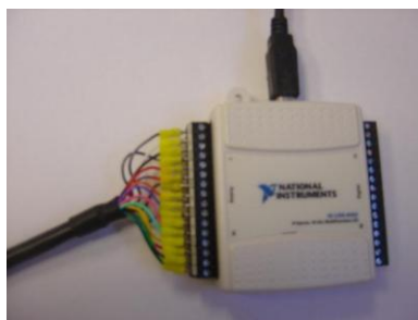
Figure 62 DAQ device used to collect PEM fuel cell data.
