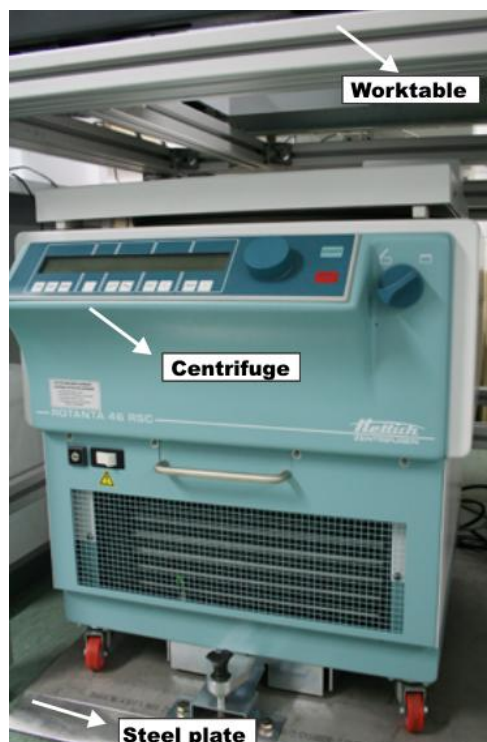
Figure 3.2.1 Centrifuge is raised with the addition of a steel plate. The centrifuge was raised by placing a steel plate underneath the instrument. This enabled the centric robotic arm to place 384 MPs into the centrifuge.
