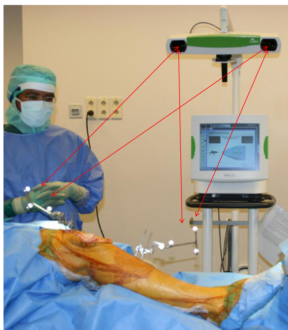
Figure 1 Infrared rays are reflected from reflection balls attached to the tibia and femur and back to the camera and the computer. The reciprocal distances and movements measured between the balls are registered by the computer which builds a model of the extremities axes and anatomy. Surgical instruments are navigated according to the same principle.
