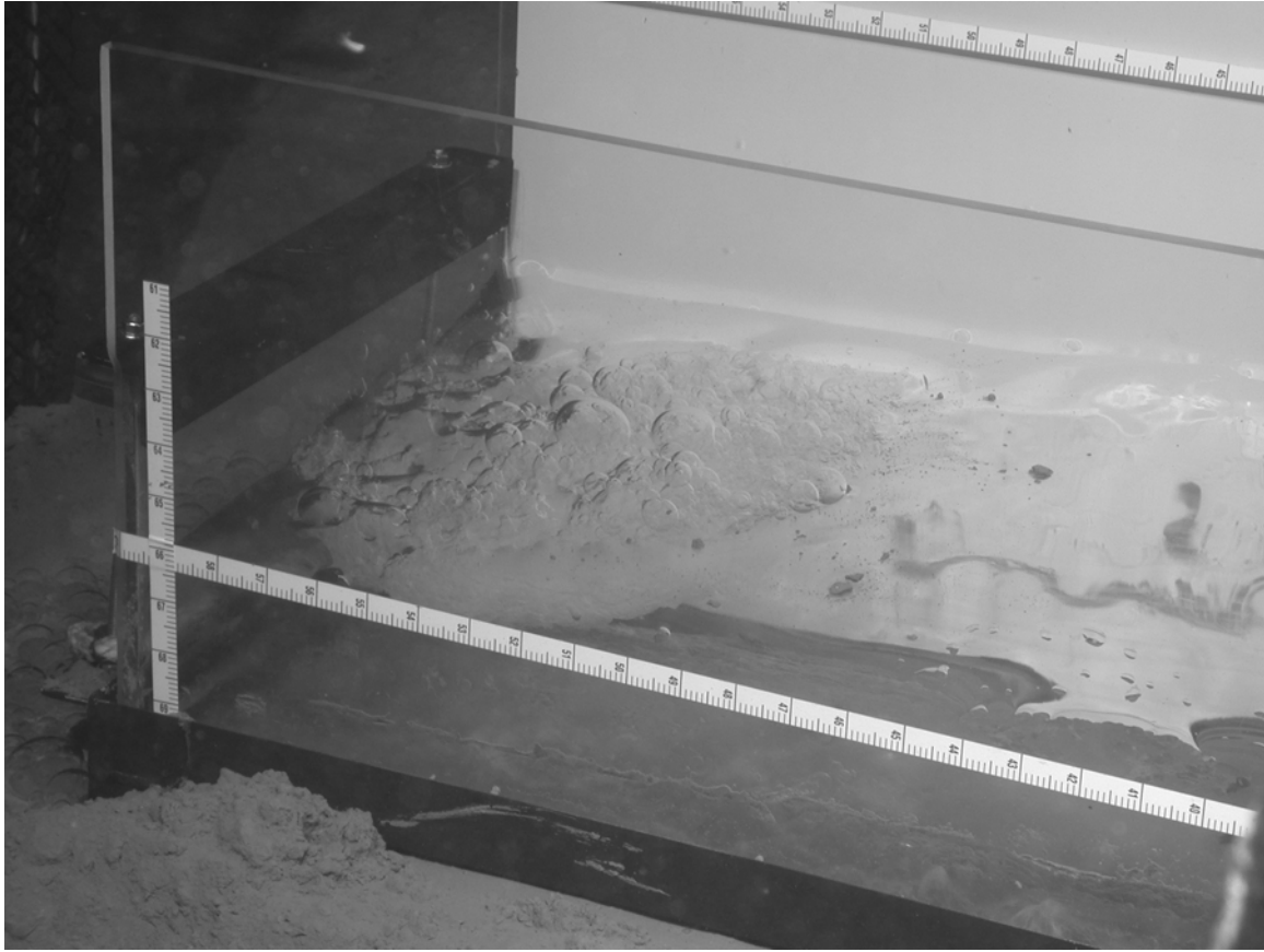
Figure 2: a) Upstream end of the trough when placed on the ocean floor at 3942 m; the thruster that produces controlled water flow can be seen at the upper right, with the mechanical wave-maker below it working directly on the endwall of the trough; b) using dye to visualize the water motion in a case with wave perturbation of the CO 2 -seawater interface; some sediment and the floating "ice" can be seen in addition to the wave pattern; c) focus on the consolidated solid downstream.
