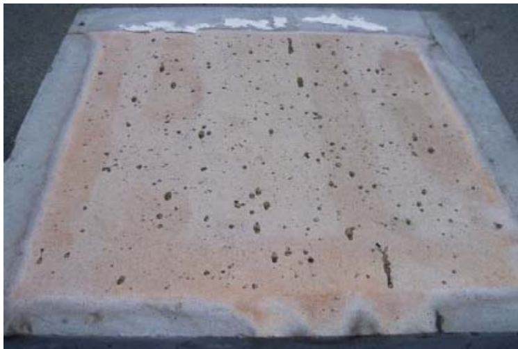
Figur 7 Lettbetong (skumglass) m/PP fiber eksponert for brann
