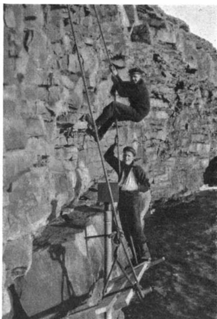
Fig. 2. Tide-gauge erected in Austervåg, Bear Island.
