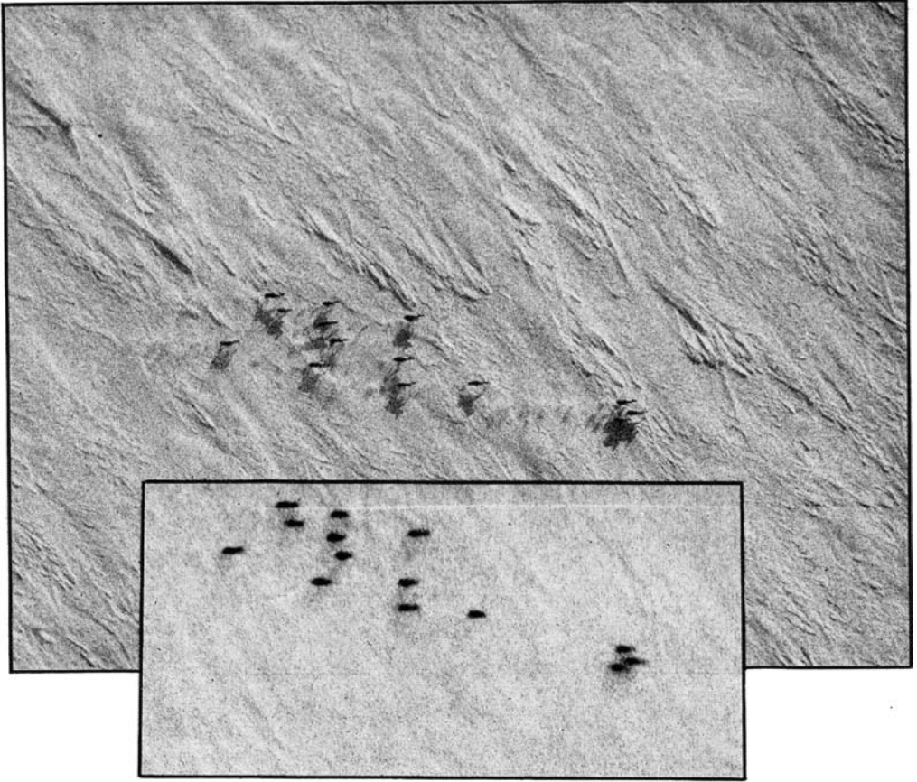
Fig. 13. Caribou Rangifer tarandus south of Churchill, Manitoba. The large black and white photograph is an enlargement from a 9 \times 9 vertical photograph taken from 450 m. The animals and their shadows are seen clearly. The insert shows an ultraviolet photograph of the same animals. Note that the shadows and details of the background have been lost, leaving only the dark shapes of the animals. Since shadows tend to mask individual animals (e.g. note the lower animal in the leading group of three), it would appear that ultraviolet photography might be useful when censusing a dense herd of caribou against a white background of snow. Elimination of shadows eases the counting of individual animals.
