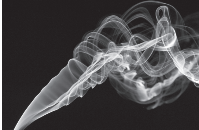
Figure 2.1: Warm smoke rising in surrounding air, visualizing the transition from laminar to turbulent flow. Photo courtesy of Jan Olav Langseth, Norwegian Defence Research Establishment .
