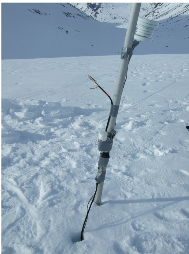
Figure § 2.4: Thermistors line and Hobo external temperature data logger mounted on stake H13.
