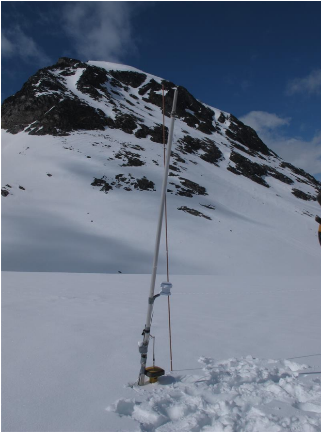
Figure § 2.8: Stake georeferencing on Hellstugubreen using DGNSS. The accuracy of the measurements may be altered by multipath effects.
