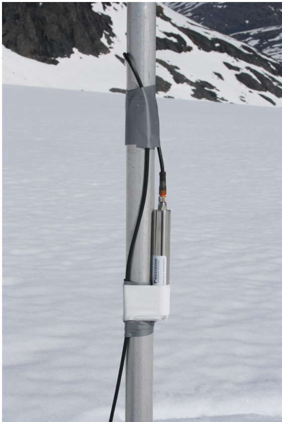
Figure § 2.6: Digital thermistors string and GeoPrecision M-Log5W data logger mounted on stake S2.
