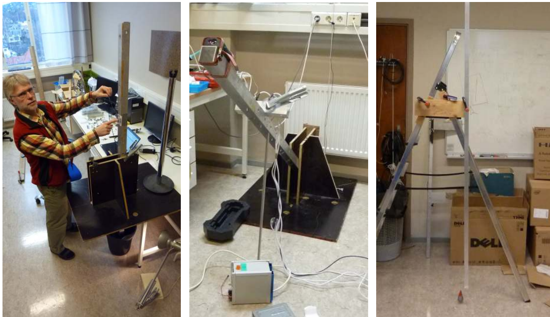
(a) Vertical reference, using a string and a heavy mass. (b) Aluminium bar with UUT. (c) Vertical ruler.
