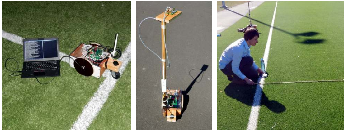
(a) Setup used to find the coordinates for the waypoints. (b) Land rover with elevated compass. (c) Measurement setup to find stone positions.
