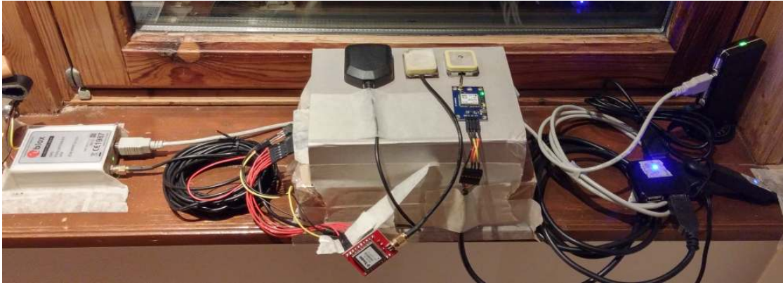
Figure 3.14: The indoor stationary GNSS-receiver test setup. The gray box to the left is the U-blox 6 PPP evaluation kit with the black antenna. The red PCB is the Trimble Copernicus II with the beige antenna in the middle. The blue PCB is the U-blox NEO-6M with the rightmost beige antenna.
