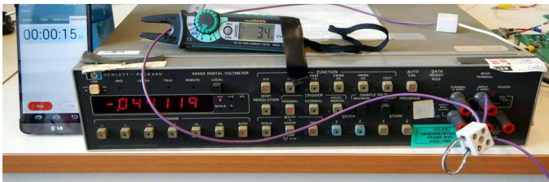
Figure 1.38: Current measurement setup for the temperature test. The power resistor is visible to the right.
