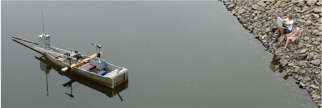
Figure 1.35: Remote controlled survey vessel supervised by operators at the shore.
