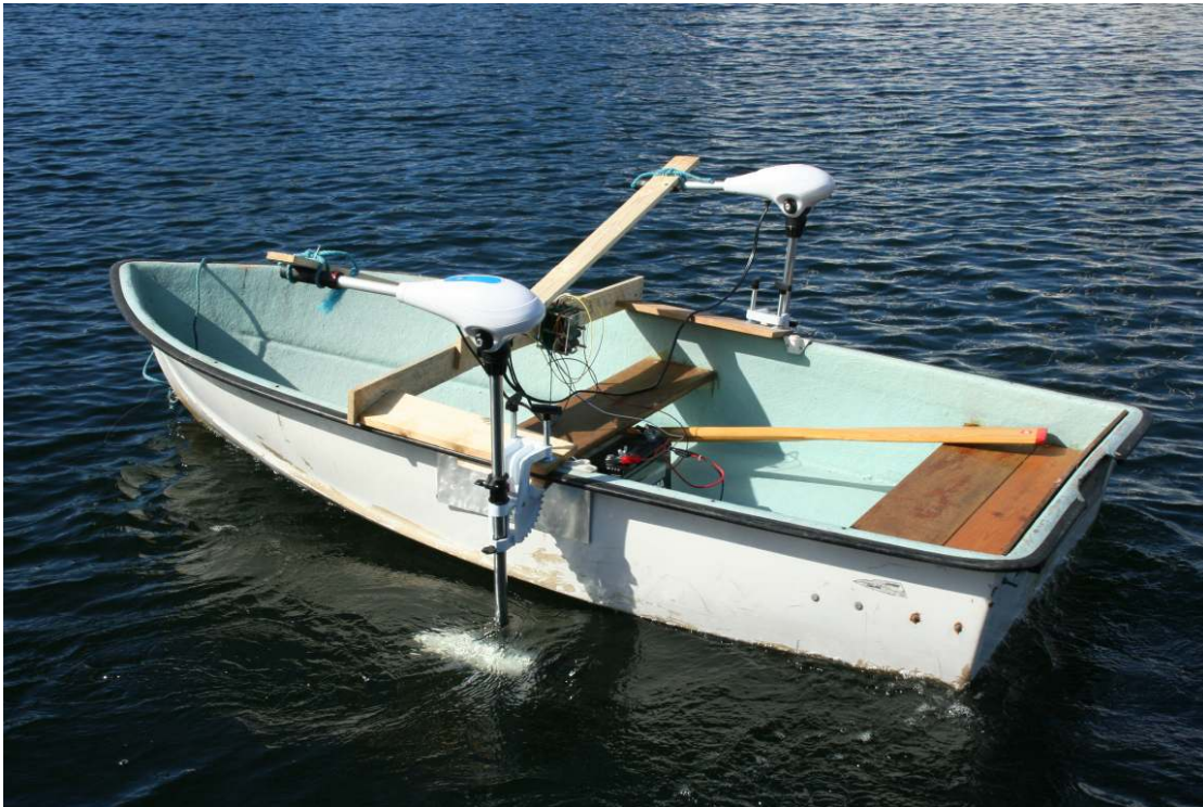
Figure 1.31: Photograph of boat, with electric engines and control unit, tested at Lysaker in May 2013.
