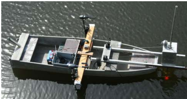
(a) Photograph of boat with a Simrad EK60 GPT.
