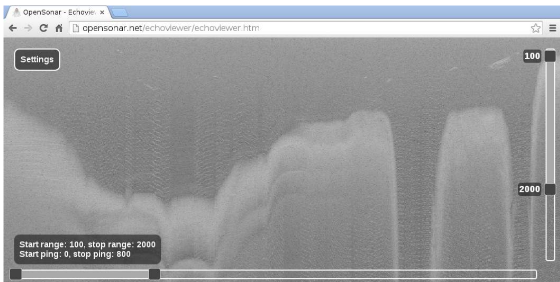
Figure 1.36: Recording from one of the test surveys conducted on lake Římov. Noise is visible as horizontal lines.
