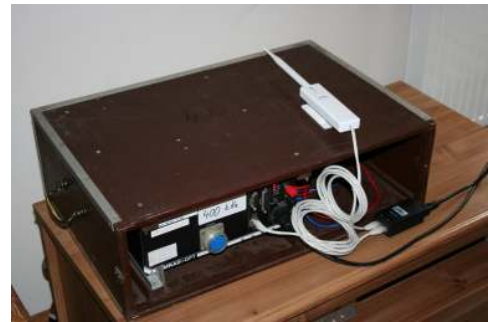
(b) Simrad EK60 GPT directly connected to a Ubiquity PicoStation M2 (through a POE-injector).
