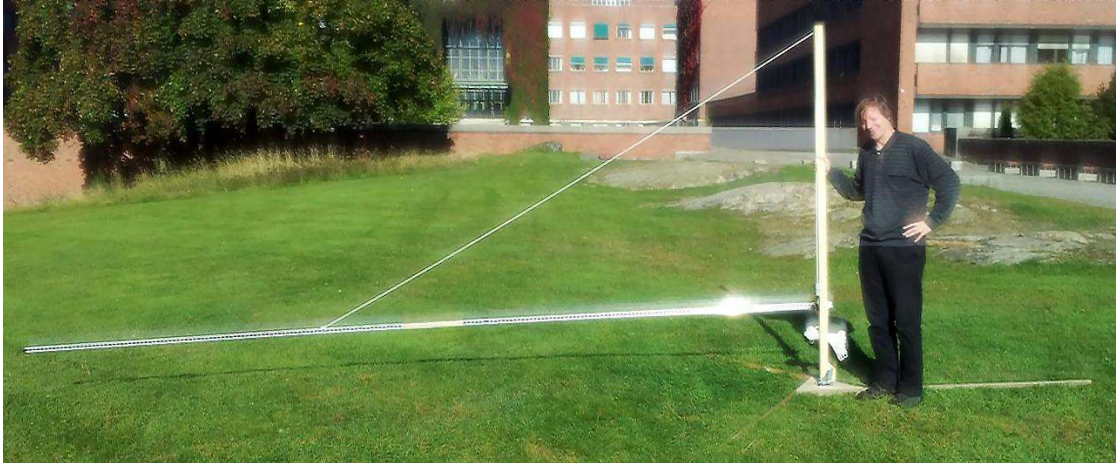
Figure 3.10: Carousel used in the moving GNSS-receiver test. The antenna of the GNSS-receiver is placed at the end of the horizontal beam. Joakim Myrland is standing next to it for scale.
