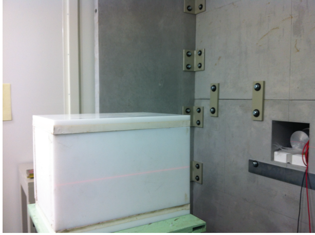
Figure 3.11: The ^3\text{He} neutron detectors are embedded in the white polyethylene in front, and a NaI detector is located in the wall behind.
