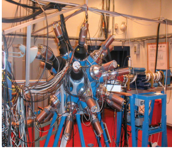
Figure 4.3: A picture of the \gamma -detector array, named CACTUS. The 28 NaI detectors are seen mounted on the outside of the sphere.
