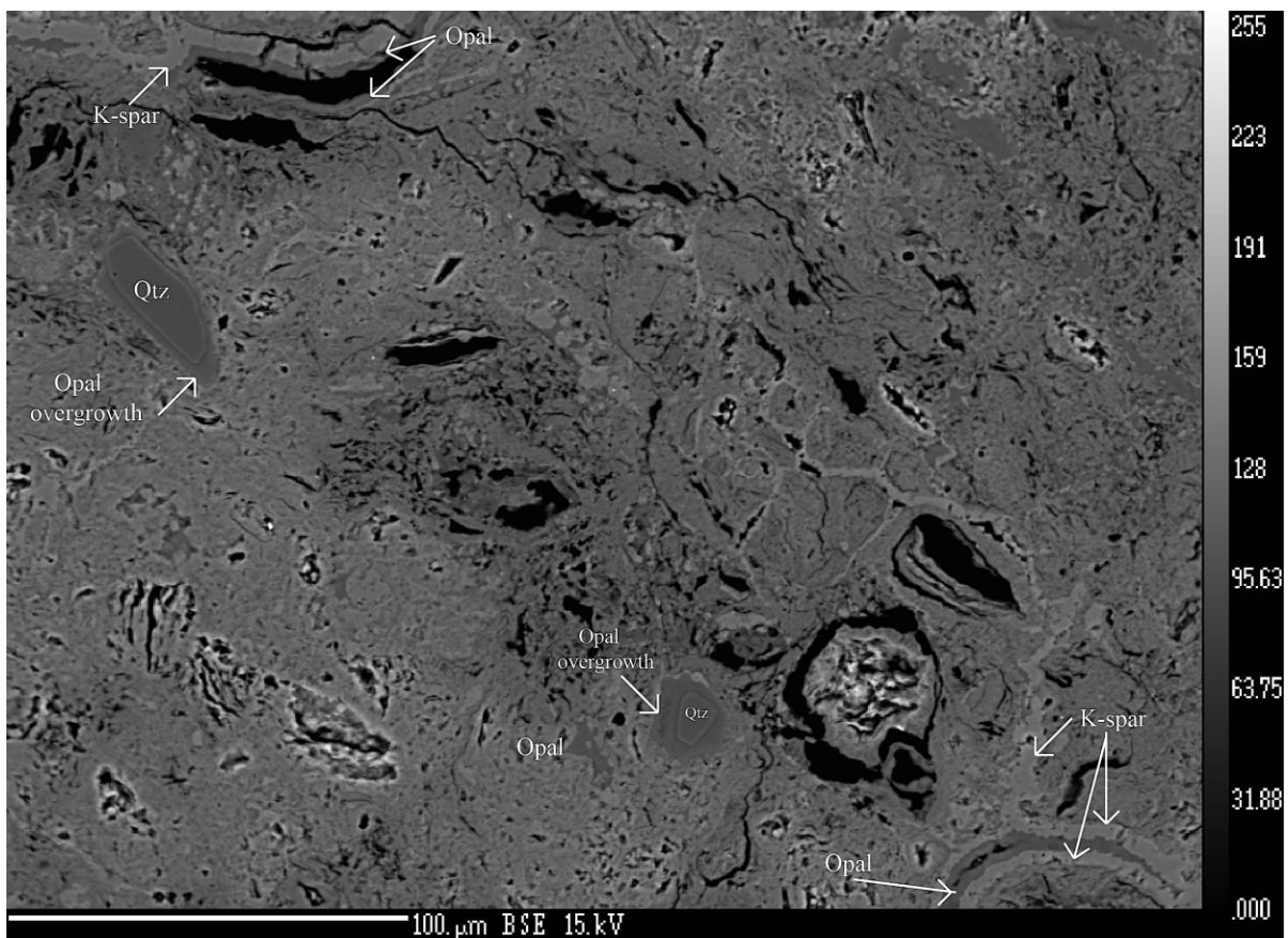
Figure 3.16 Electron microprobe analysis of SARP 2-10. The matrix is composed of k-spar and opaline silica. Overgrowth by opaline silica on quartz grains have been detected
