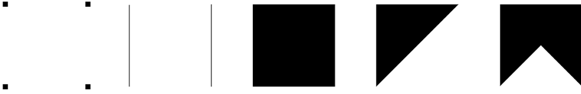
Figure 10.1: The vertices \{(0,0), (0,1), (1,1), (1,0)\} have been rendered as the primitives (from left) GL_POINTS , GL_LINES , GL_TRIANGLES , GL_QUADS and GL_TRIANGLE_STRIP . We see that the final rendered geometrical objects are quite different for the different primitives.
