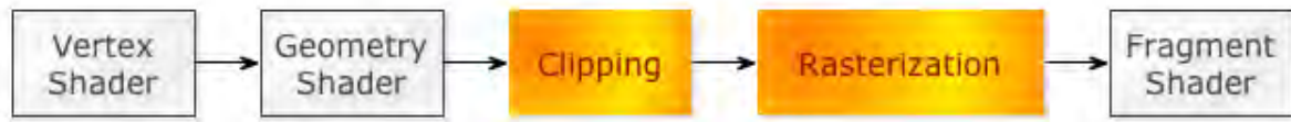
Figure 10.6: Diagram of the OpenGL rendering pipeline. The gray boxes are shader steps (the shader programs can be written by the user). Each vertex is processed in the vertex shader before it is sent to the geometry shader that can create zero or more vertices based on the input vertex. Each vertex is then analyzed in the clipping program that removes vertices that cannot be rendered. The rasterization program creates a two dimensional image of every triangle so that the fragment shader can merge everything to color values per pixel on the screen. Not that the full pipeline contains more steps, but these are the relevant stages for understanding what our visualization tool does.
