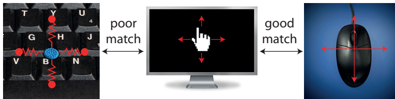
Figure 2.4: The mouse is better perceptually understood as a position marker mover than the pointing stick on a laptop. This is because the match between control space and output space is better.
