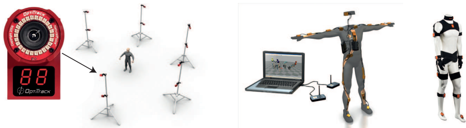
Figure 3.4: The two main MoCap systems that have been used during the work of this thesis are the OptiTrack V100:R2 (left) and the Xsens MVN system (right). Notice the IR LEDs on the OptiTrack camera which are used as the light source to light up reflective markers. The strap-on suit, on the far right, is the Xsens suit we have used for the Dance Jockey project.
