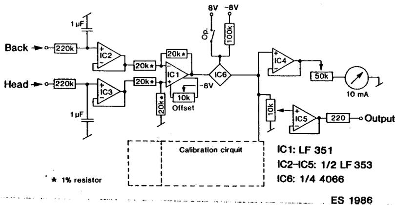
Figure 3: Electric diagram for continuous calculation of the neck angle from the head and back angles. The calibration circuit is identical to the one shown in figure 2.
