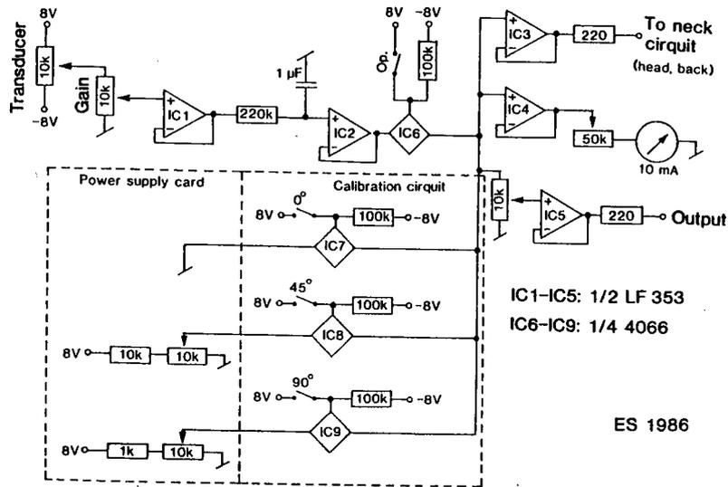
Figure 2: Electric diagram of the "Ergonometer" for head, arm and back angles. An electric calibration circuit is shown within the interrupted lines. The RC-circuit between IC1 and IC2 sets the time constant to about 0.2 s.
