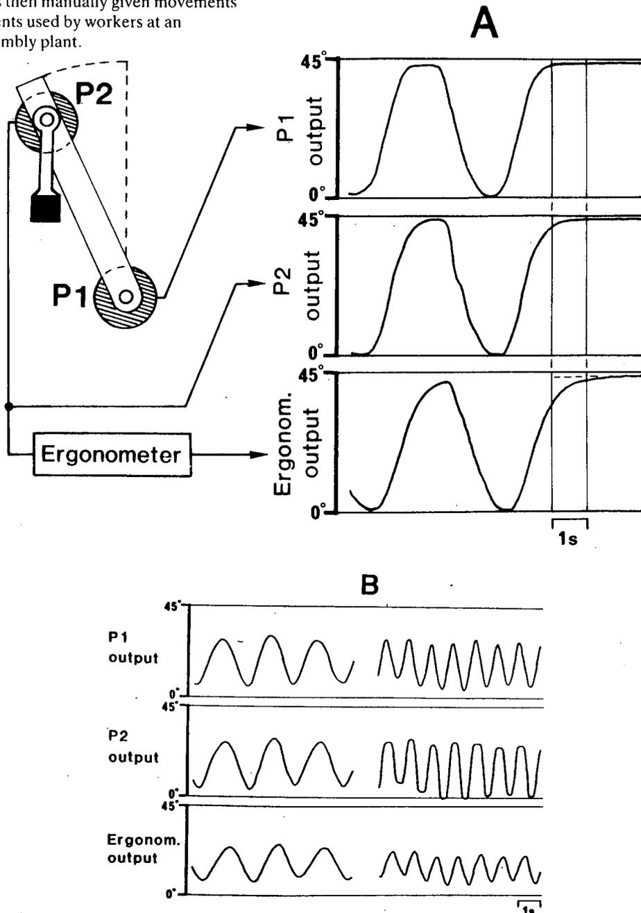
Figure 6: In vitro test setup for determination of the pendulum transducer characteristics (P2 output) and output from the "Ergonometer" (Ergonom. output) as compared to true angular movement of the transducer (P1 output). A: A stepwise movement indicates the time delay by the "Ergonometer" caused by the inherent electronic time
