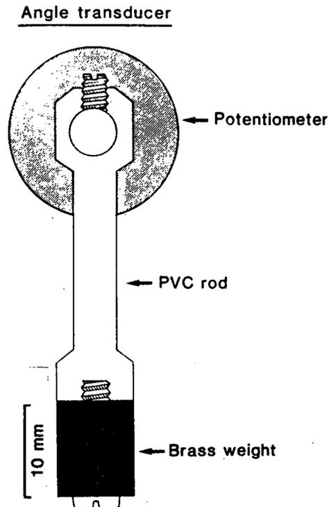
Figure 1: Schematic illustration of the potentiometer pendulum transducer. A standard Spectrol Model 157 potentiometer with a pendulum attached to the axis is used. In later versions ball bearings are applied to reduce the rotational friction.
