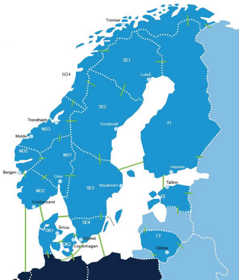
Figure 1.1: Nord Pool Spot price areas as of January 2013. The green lines denote possible flows between the price areas. Source: http://www.nordpoolspot.com/
