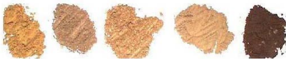
Figure 9: Illustration of the appearance of Reverse Osmosis (RO) isolated samples of DOM.
