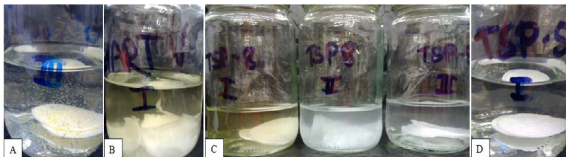
Figure 20: Photos illustrating the different appearance of the sample solutions which developed throughout the course of the biodegradation experiment; A) development of what described as suspended particles, B) opaqueness of the sample solution caused by disintegration of the added glass fibre filters, C) difference in the appearance of three sample replicates of one sample, and D) no visible change in the appearance of the sample solution. Note that the brownish-colour of the sample solution in figure B is caused by the DOM.
