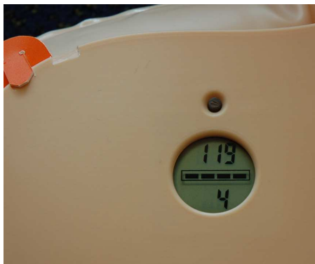
Figure 3. The MiniAnne counting device. The number of correct chest compressions (top) and mouth-to-mouth ventilations (bottom) during the first two minutes of BLS.
